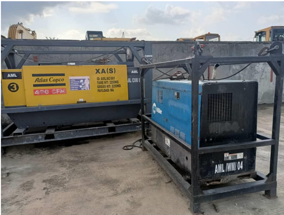
AIR COMPRESSOR AND WELDING MACHINE
